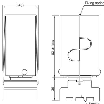
State in which the fixing spring is mounted
