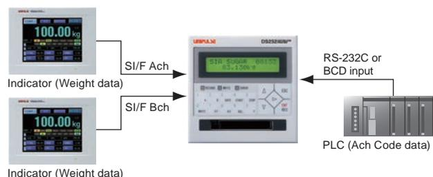
By entering via the front panel key, weight data with code can be recorded in both A ch and B ch. Code data of A ch can also be entered via an optional interface.
