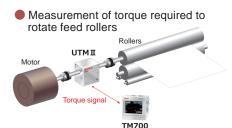
Torque fluctuation can be monitored while a sheet of paper or film is fed by the drive roller.
