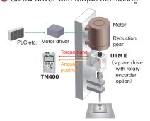
Torque can be measured in the process of tightening screws. Since the torque can be controlled during the whole process, the system can be applied to automation of process.
