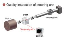
By measuring the torque required to rotate automotive parts such as steering unit, it is possible to quantize the smoothness of the rotation for standardization of the quality inspection
